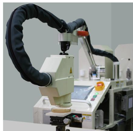
Fig. 1: The generator of low temperature argon plasma
