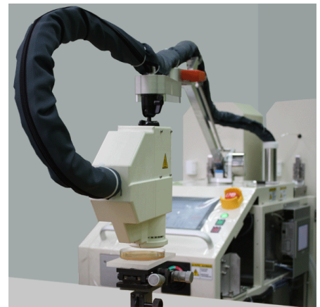
Fig. 1: The generator of low temperature argon plasma
