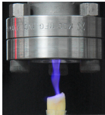
Fig. 2: The room temperature plasma jet impinging into a root canal
