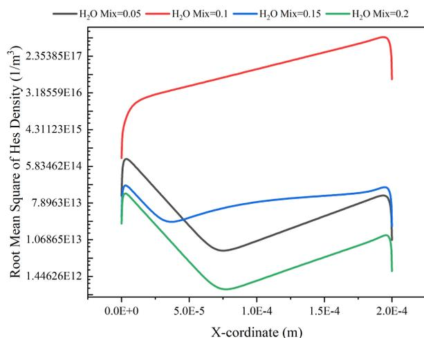
**Figure 9.** The spatial distribution of the exited helium density for different percentages of H<sub>2</sub>O at sh = 0.05, 0.1, 0.15, and 0.2.
