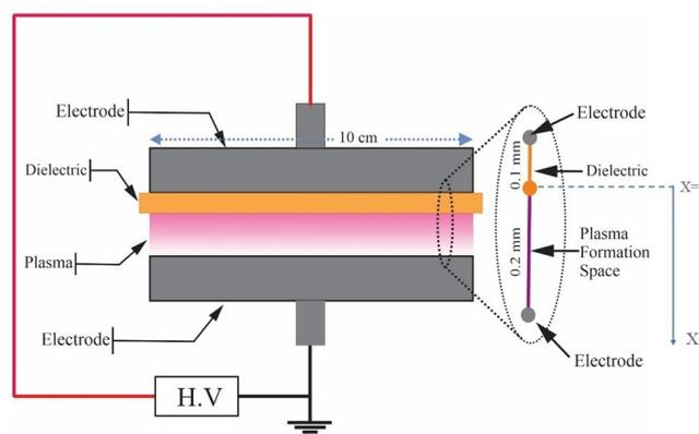
**Figure 1.** A schematic of the structure of the plasma by presenting the locations of the electrodes on the surface and inside of the behind dielectric.
