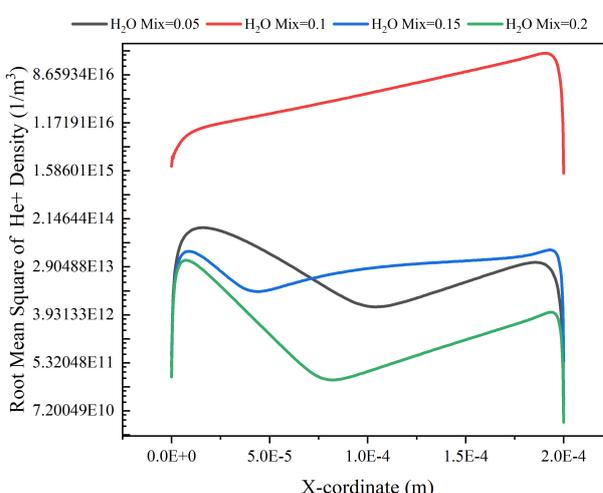
**Figure 8.** The evolution of  $He^+$  density versus distance, for different percentages of  $0.05, 0.10, 0.15,$  and  $0.20$ .
