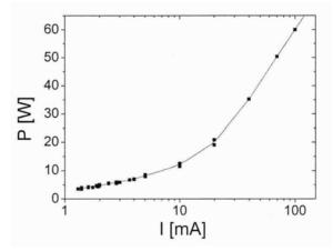
**Figure 3.** Discharge power as a function of current. Interelectrode distance d = 7 mm.
