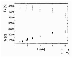
Figure 5. Rotational and vibrational temperatures as functions of the discharge current in ambient air at low flow velocity  $v \approx 0.2$  m/s, interelectrode distance d = 7 mm.
