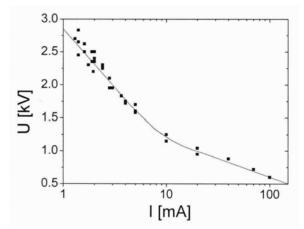
**Figure 2.** Voltage-current characteristic of the DC discharge in ambient air. Interelectrode distance d = 7 mm.
