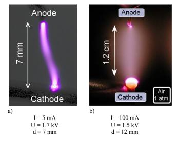
**Figure 4.** DC glow discharges in ambient air flow (v = 0.2 m/s) at atmospheric pressure (different exposure times were used).
