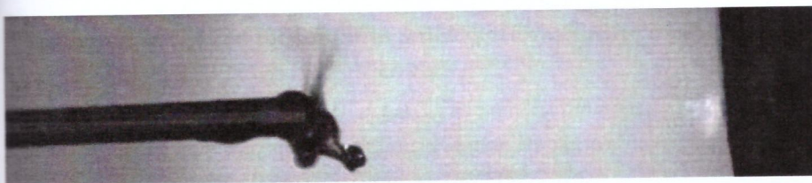
Figure 1: An illustrative image of the transient spark's interaction with water, captured by an ultrafast camera.
