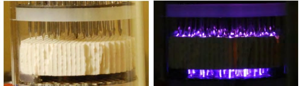
discharge in honeycomb monoliths
