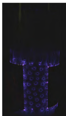
Discharge assisted by AC pellet bed discharge
