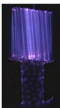
Discharge assisted by AC multi-hollow DBD discharge
